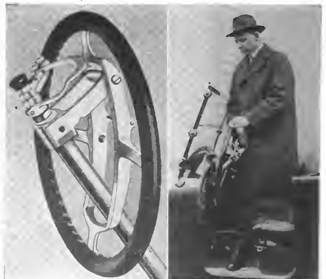
The Vincent Clear-Room Steering Wheel. Left—Detail of the wheel in the tilted position. Right—The wheel in use. Note the wide passage by the driver's seat
